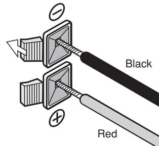
Press the button of the speaker jack and keep it pressed down as you insert the wire of the speaker cord and then release the button.
